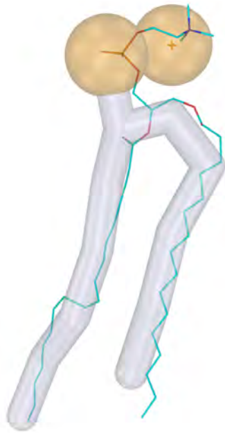
Fig. 3. Example of coarse-grained lipid compared with its atomistic structure. A 4:1 mapping is used, i.e. one coarse-grain bead represents four heavy atoms. Note that the phosphate and ethanolamine groups of the lipid are modelled by a single coarse-grained bead.
